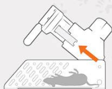
Auto-reset The pest drops as the trap resets itself
